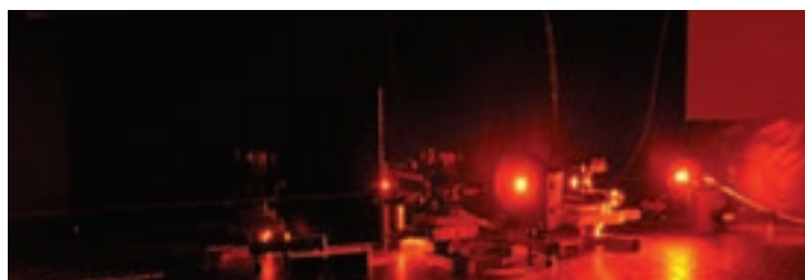
Fig. 1: Picture of a frequency doubled VECSEL operating at 620 nm.
