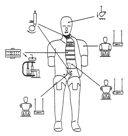
$\label{eq:Figure 4} \textit{Figure 4}$  Neck and lumbar spine certification test set-up
