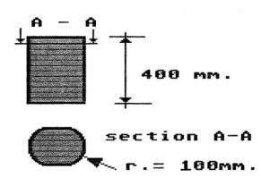
FIG. 3 body block impactor
