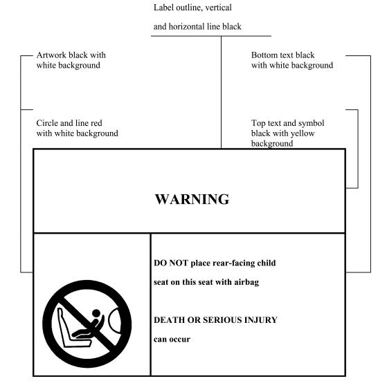
The overall dimensions shall be 120 x 60 mm or the equivalent area, as a minimum.
