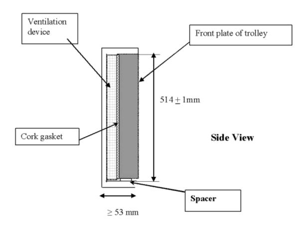
$\label{eq:Figure 6} \textit{ Attachment of backplate to ventillation device and trolley faceplate}$
