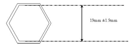
$\label{eq:Figure 4} \mbox{Dimension of aluminium honeycomb cells}$   $\mbox{Design of the back plate}$
