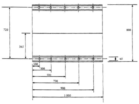
Hole diameters 9,5 mm. All dimensions in mm.
