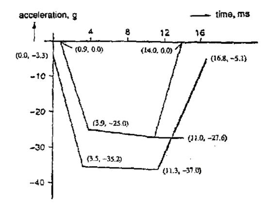
$\label{eq:Figure 6} \textit{Figure 6}$  Pendulum deceleration-time corridor for lumbar spine certification test
