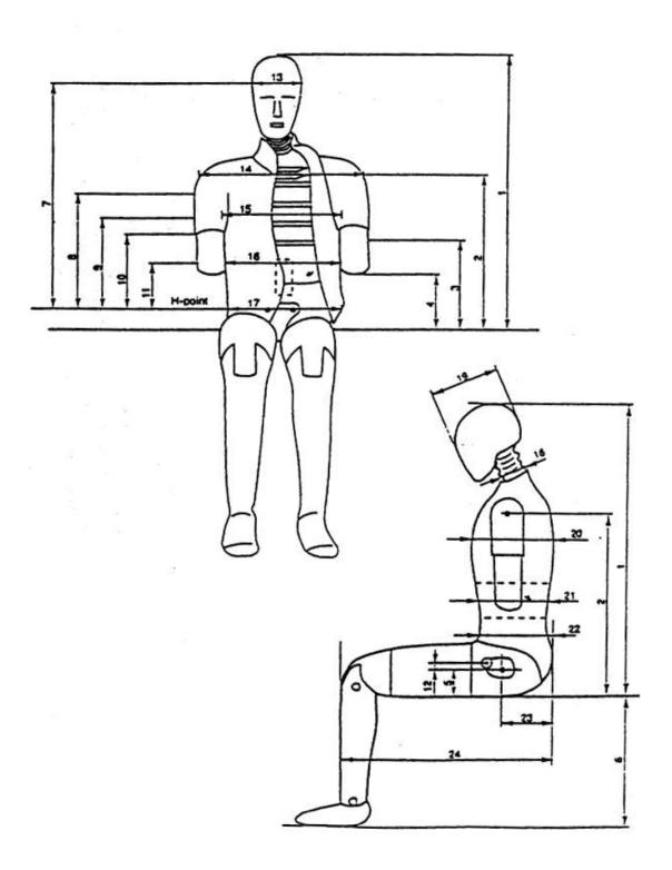
Figure 2  $\label{eq:Figure 2}$  Measurements for principal dummy dimensions  $\mbox{(See Table 3)}$
