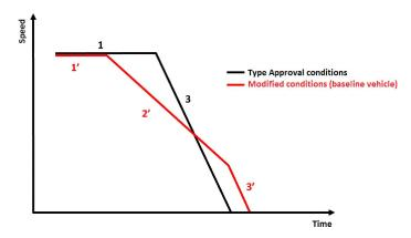
A common characteristic of a baseline vehicle is that, during deceleration phases of the type approval (NEDC) (3) and modified (2' + 3') testing conditions, no fuel is used (cut-off).
