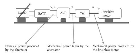
$\begin{array}{lll} TM &=& Torquemeter \\ ALT. &=& Alternator \\ BATT. &=& Battery \\ V,I &=& Volt, \ current \\ T &=& Torque \\ \omega &=& Rotational \ speed \\ \end{array}$
