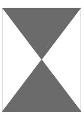
The lamps or plates must be on the same height above buffer on the transversal axis. Member States that require 2 reflective plates must also accept 2 steady red lights as train rear end indication.
