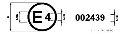
The above approval mark affixed to a pneumatic tyre shows that the type of tyre concerned has been approved in the Netherlands (E 4) under approval number 002439. The first two digits of the approval number indicate that the approval was granted in accordance with the requirements of Regulation No 54 in its original form.
