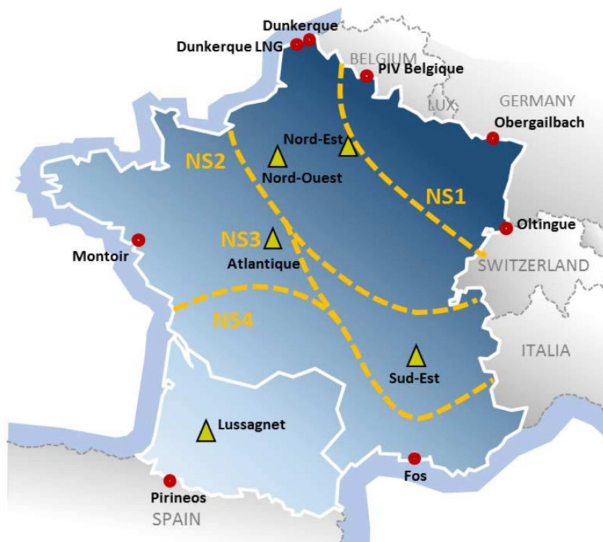
Figure 1: Main operational limitations likely to be observed in the transmission network when suppliers seek to maximise natural gas injections from north-eastern France
