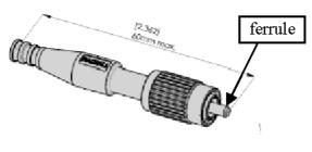
The ferrule is the most important component in terms of the connector's operation and may be made of ceramic, zirconium oxide (ceramic), nickel silver, glass, tungsten carbide, etc. Though the material of the ferrule does not normally predominate in the connector as a whole, the importance of the ferrule to the product's application is such that the material is to be seen as determining the connector's essential character.
