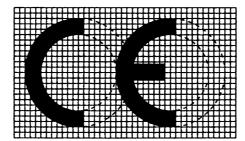
If the CE marking is reduced or enlarged, the proportions given in the above drawing must be respected.
