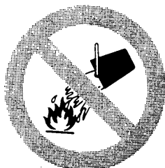
Do not extinguish with water
