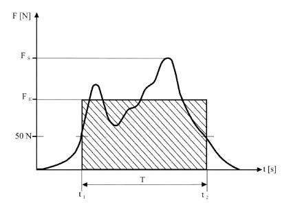
2.6. Clamping or mean reactive force  $F_C$  is the arithmetical mean value of the effective forces, measured at the same measuring point subsequently more times:
