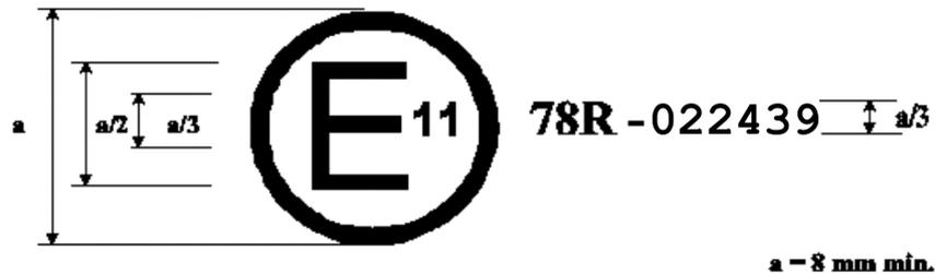
The above approval mark affixed to a vehicle shows that the vehicle type concerned has, with regard to braking, been approved in the United Kingdom (E 11) pursuant to Regulation No 78 under approval number 022439. The first two digits of the approval number indicate that Regulation No 78 already included the 02 series of amendments when the approval was granted.
