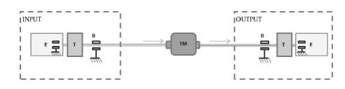
E: Electric machine T: Torque sensor B: Bearing TM: Transmission
