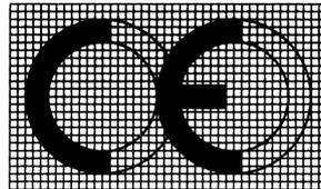
If the CE marking is reduced or enlarged, the proportions given in the above graduated drawing must be respected.
