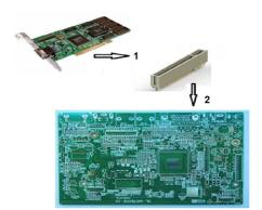
**1**: This connector is not intended to be directly attached to a PCB and is therefore excluded from this subheading. **2**: This connector is intended to be directly attached to a PCB and is therefore included within this subheading.'
