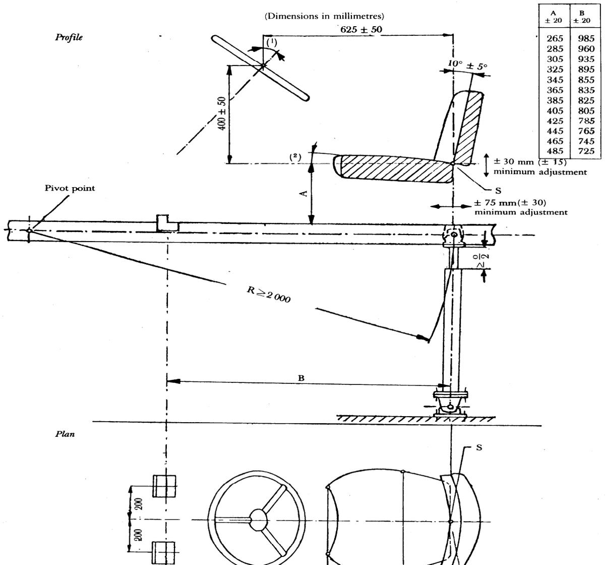
(1) The angle of the steering column in relation to the vertical depends on the position of the seat, the diameter of the steering wheel.
