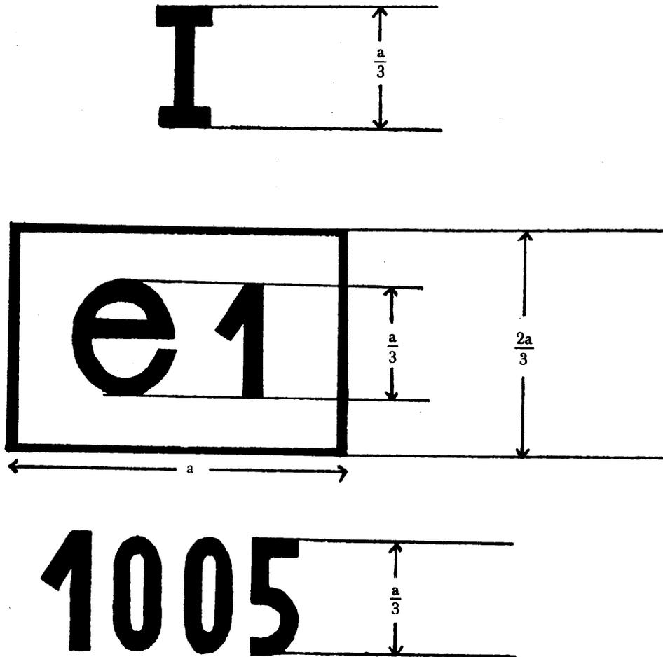
The seat bearing the EEC EC type-approval mark above is a seat intended for a Category A tractor in Class I and approved in Germany (e1) under number 1 005.
