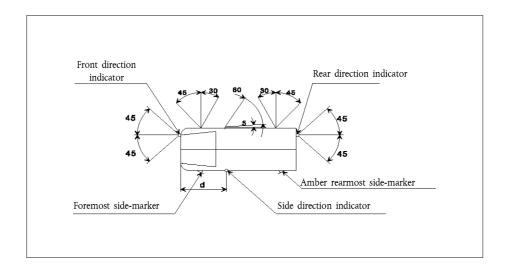
Vertical angles: 15° above and below the horizontal. The vertical angle below the horizontal may be reduced to 5° if the lamps are less than 750 mm above the ground.
