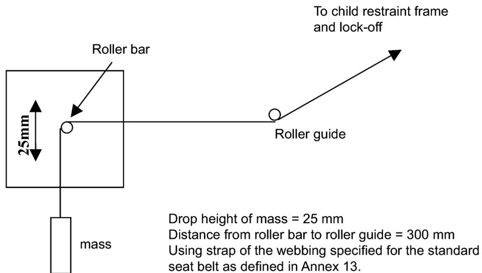
Figure 6: Schematic layout of Class B Lock-off test
