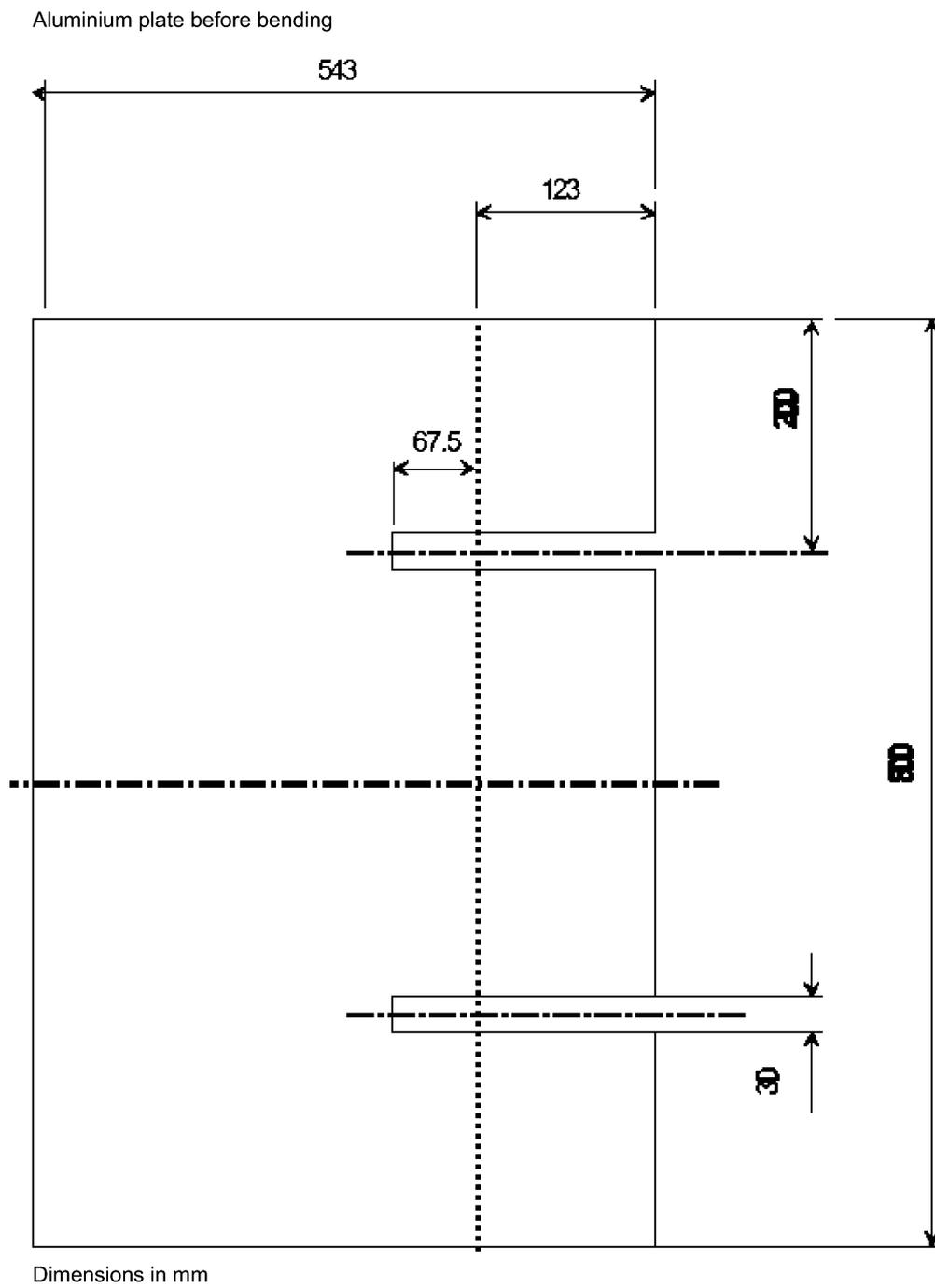
Figure 2: Dimensions of the aluminium bottom plate
