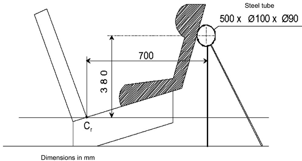
Figure 1: Arrangement for testing a rearward-facing device
