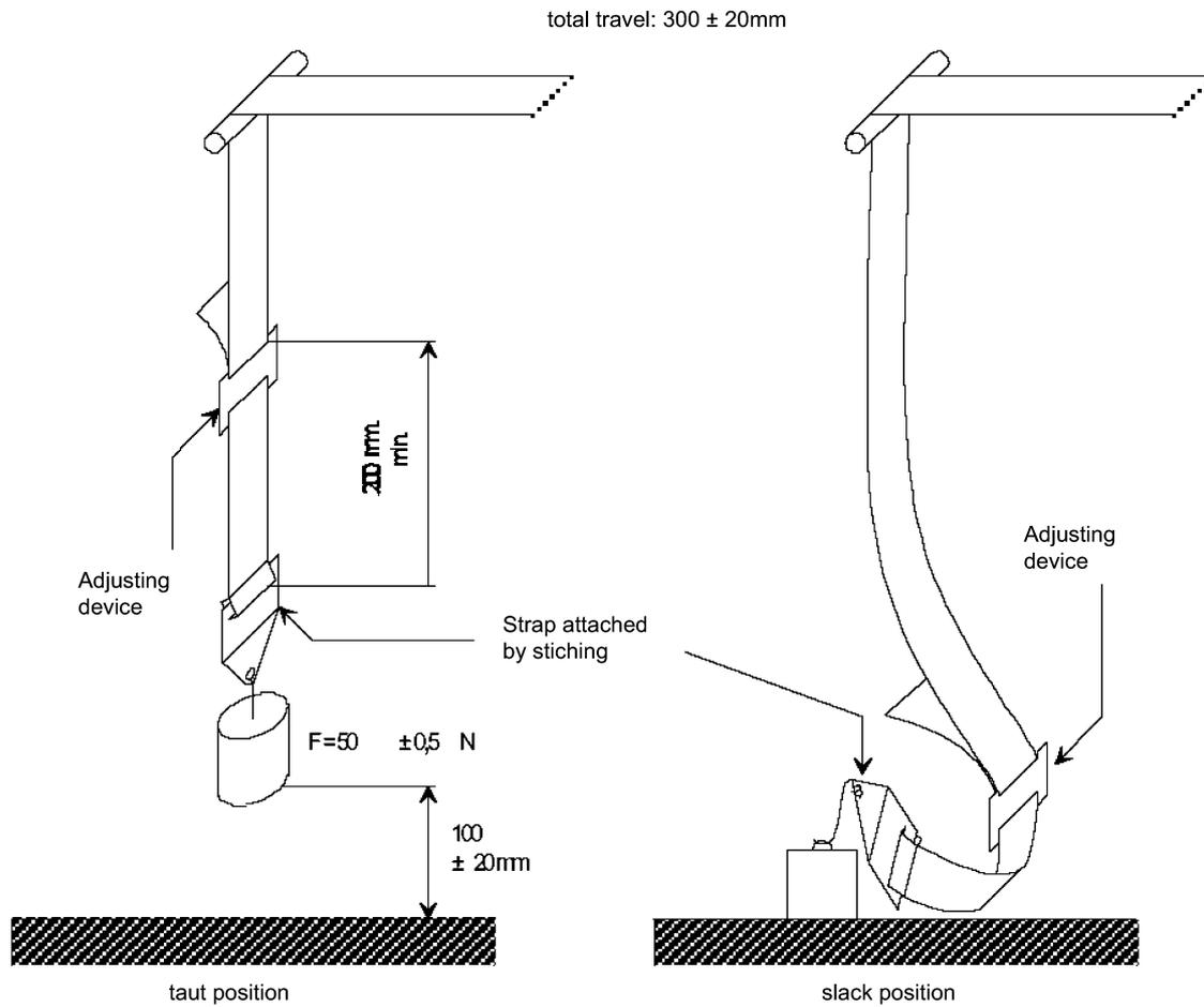
The load of 50 N on the testing device shall be vertically guided in such a way as to prevent load-swing and twisting of the strap.
