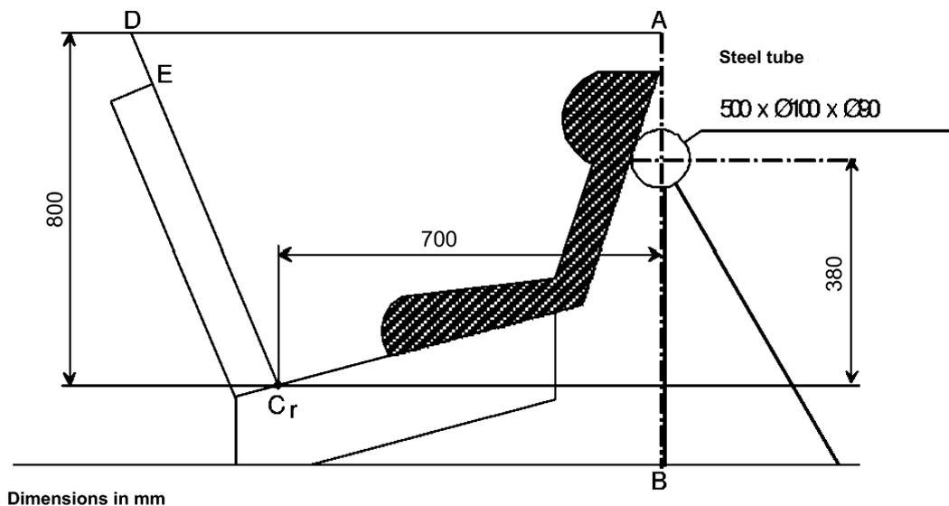
Figure 2: Arrangement for testing a rearward-facing device
