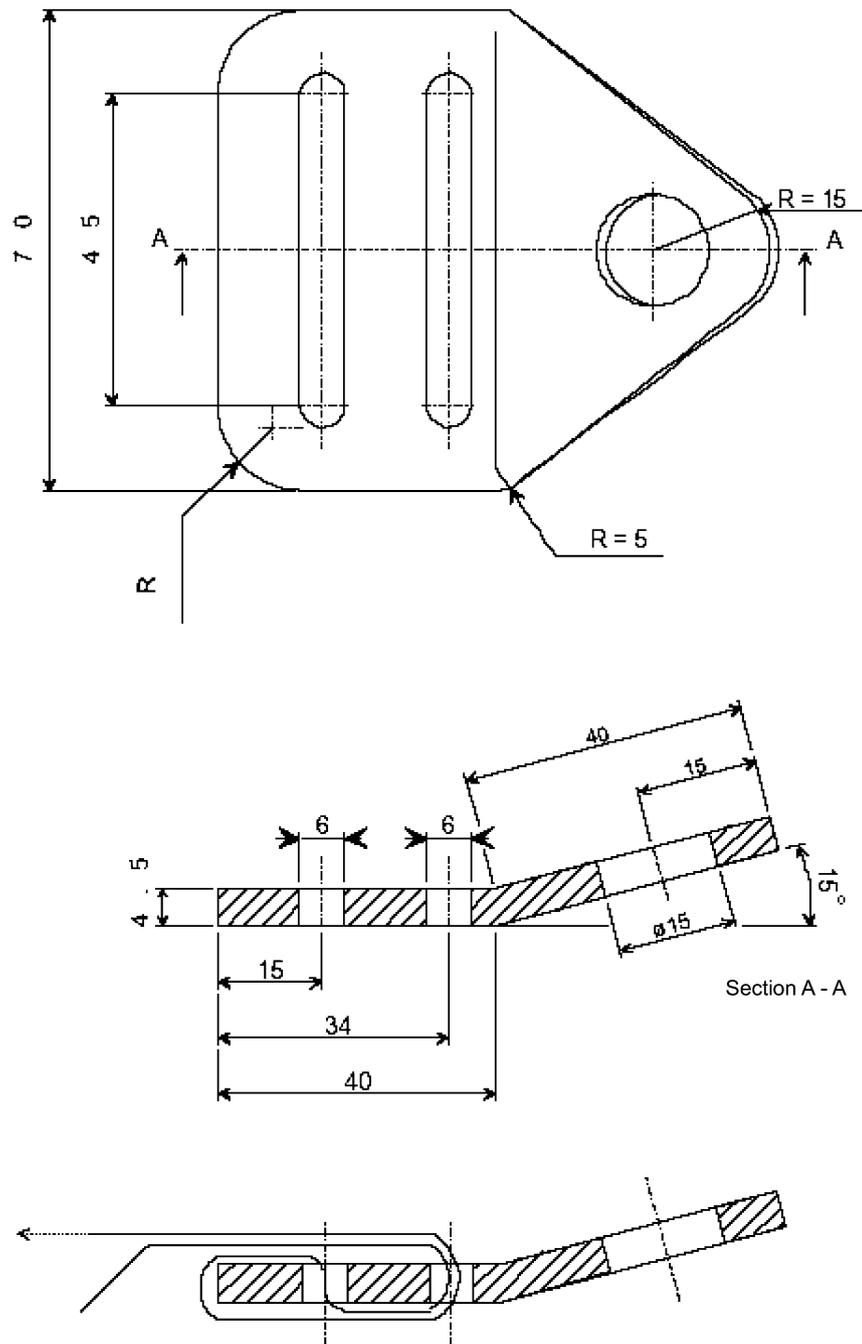
Figure 2: Typical standard anchorage plate.
