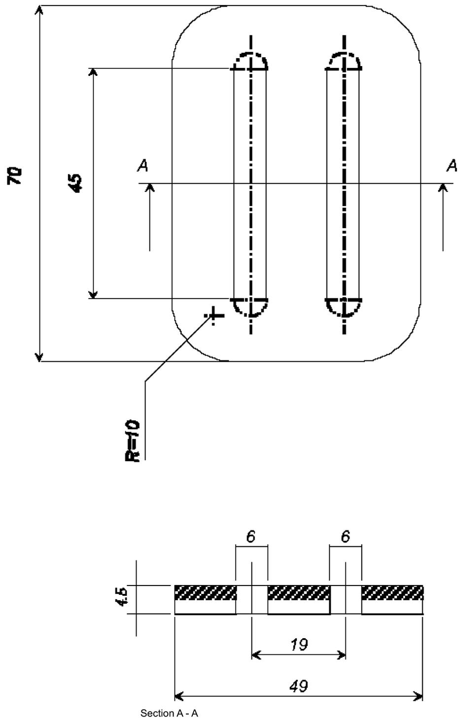
Figure 3: Central part of standard belt configuration
