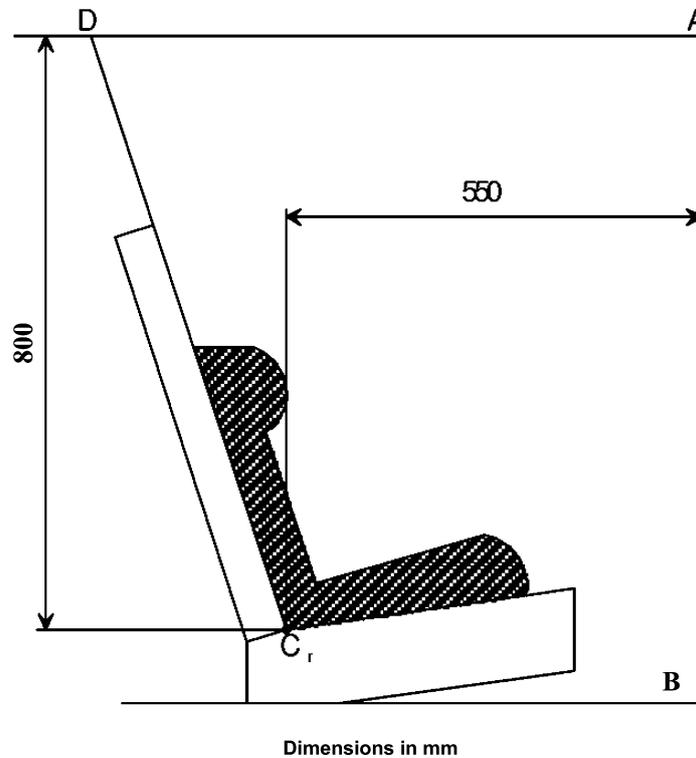
Figure 1: Arrangement for testing a forward-facing device
