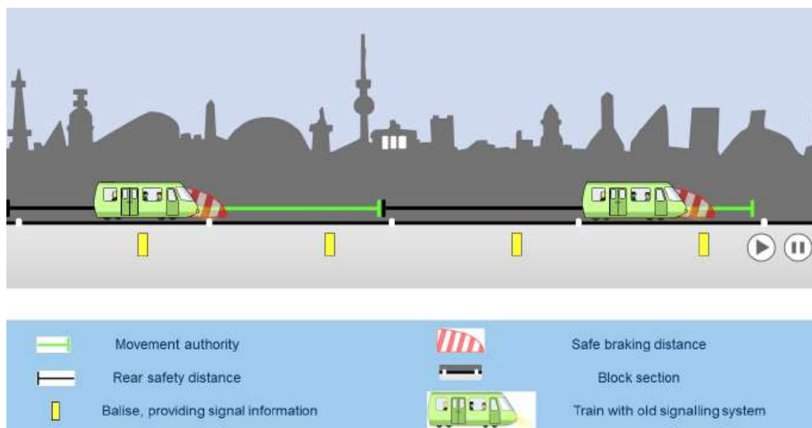
Figure 3: Urban signalling (Metro) – Conventional technology
