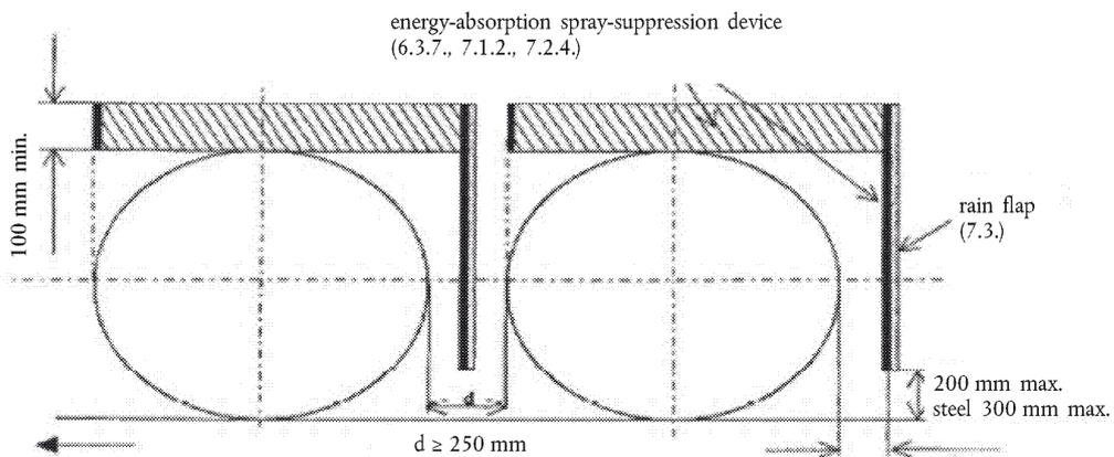
(b) Single axles or multiple axles where the distance between the tyres is not less than 250 mm.
