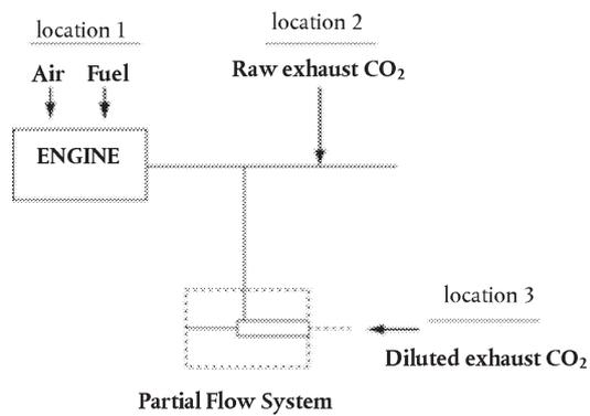
**2. Carbon flow rate into the engine (location 1)**
