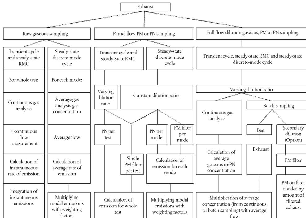
Note on Figure 6.2: The term 'Partial flow PM sampling' includes the partial flow dilution to extract only raw exhaust gas with constant or varying dilution ratio.
