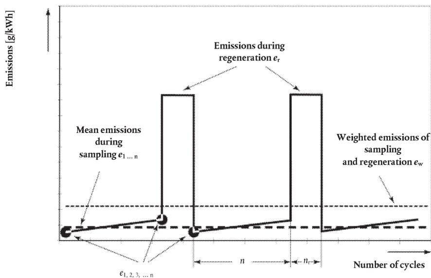
The average specific emission rate related to the test runs conducted according to points 6.6.2.1 or 6.6.2.2 [g/kWh or #/kWh] shall be weighted by means of equation (6-9) (see Figure 6.1):
