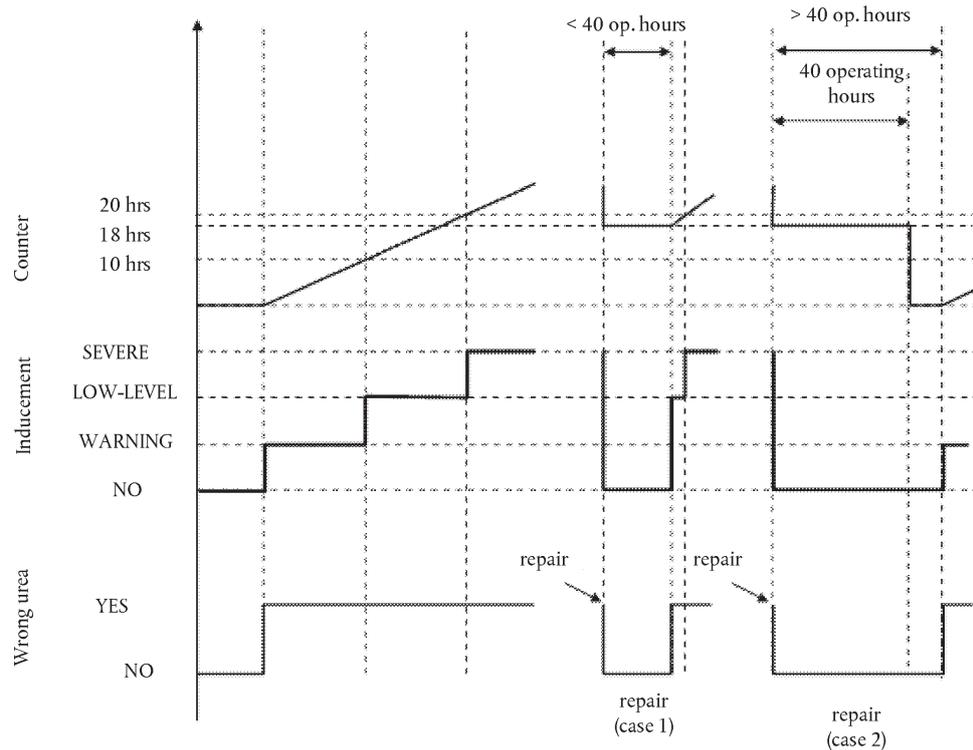
12.4. Figure 4.7 illustrates three cases of failure of the urea dosing system. This Figure also illustrates the process that applies in the case of the monitoring failures described in section 9:
