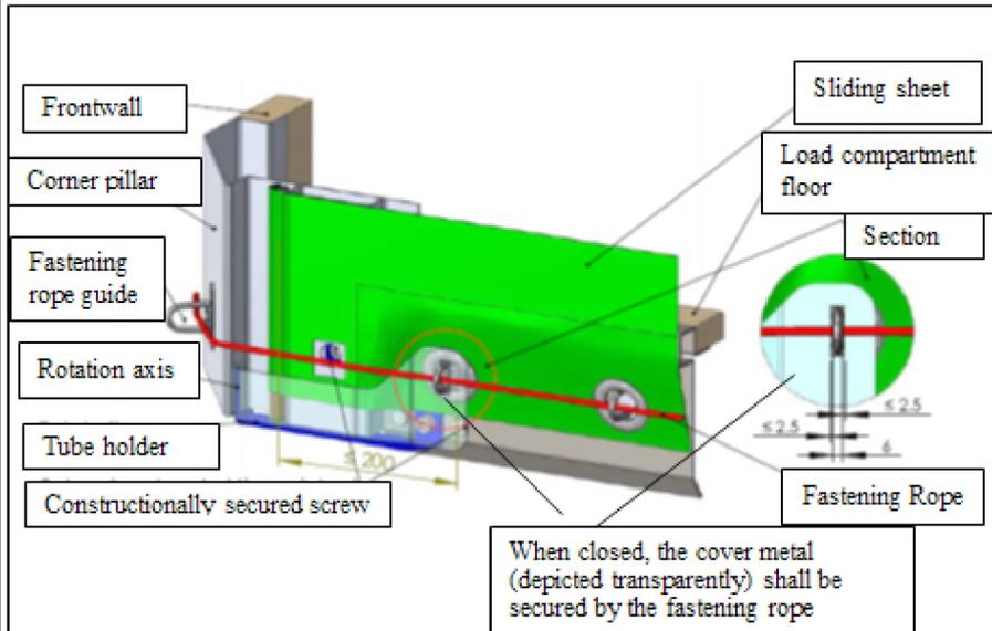
**(b) Narrow oval eyelet, anti-lifting system for the tensioning tube**
