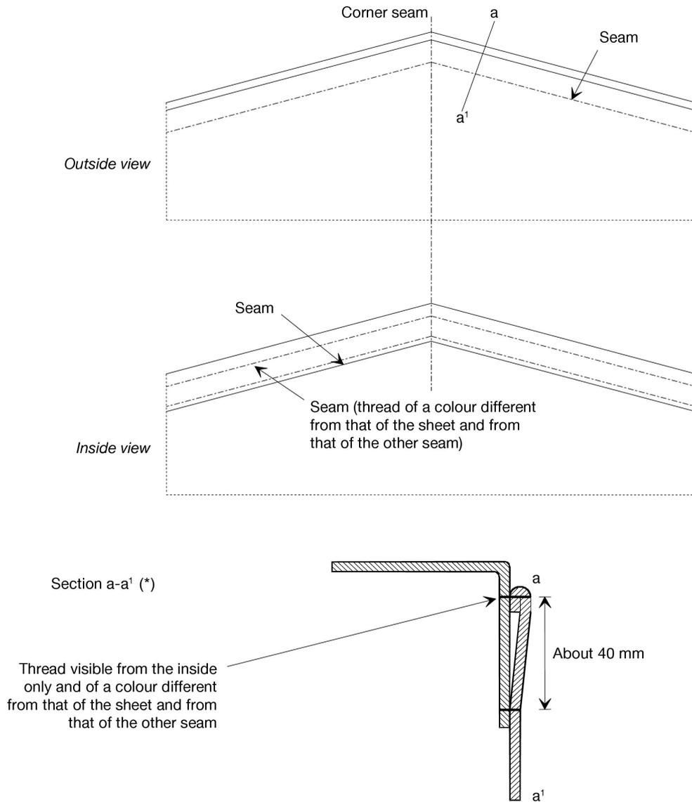
N.B. Corner seams made according to the method shown in sketch No 2a) of Annex 2 to this Convention are also acceptable.
