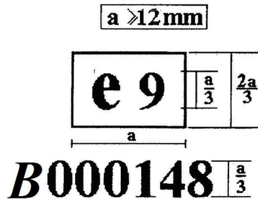
The silencing system, or components thereof, bearing the above EU type-approval mark is a device which has been approved in Spain (e 9) pursuant to Regulation (EU) No 540/2014 under the base approval number 0148, complying with the limit values of Phase 2 in Annex III to that Regulation.
