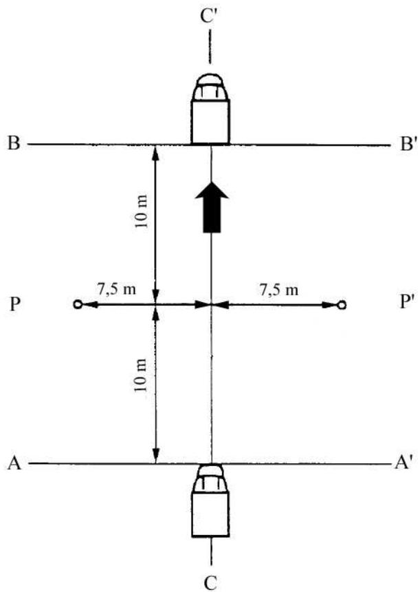
Figure 1: Measuring positions for vehicles in motion
