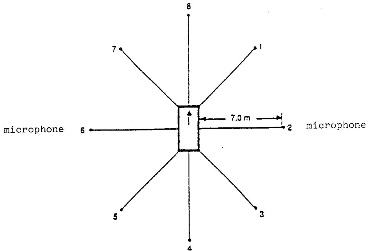
The measurement is performed at the stationary vehicle in accordance with Figure 1, using two microphone positions at a distance of 7 m from the contour of the vehicles and at 1,2 m above ground.
