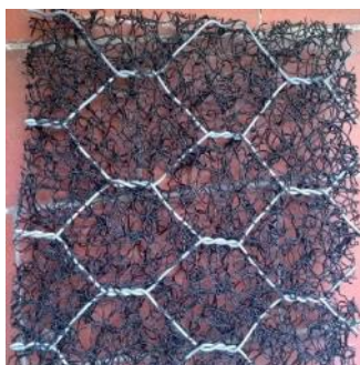
Figure 36: Geotextile mesh used for vegetation support
