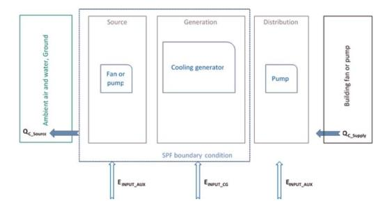
Figure 1 Illustration of SPF boundary conditions for cooling generator using standard SPF and district cooling (and other large cooling systems using measured SPF), where  $E_{INPUT\_AUX}$  is the energy input to fan and/or pump and  $E_{INPUT\_CG}$  the energy input to the cooling generator
