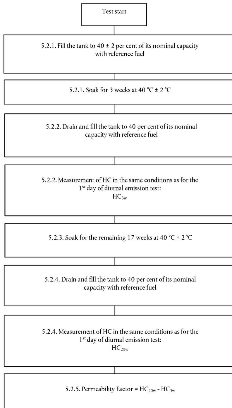
5.2.1. The fuel tank system representative of a family shall be selected and mounted on a rig in a similar orientation as in the vehicle. The tank shall be filled to  $40 \pm 2$  per cent of its nominal capacity with reference fuel at a temperature of  $18 \text{ °C} \pm 2 \text{ °C}$ . The rig with the fuel tank system shall be placed in a room with a controlled temperature of  $40 \text{ °C} \pm 2 \text{ °C}$  for 3 weeks.
