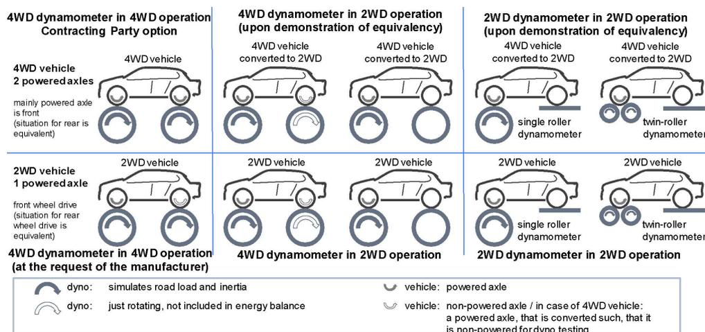
2.4.2.5. Demonstration of equivalency between a dynamometer in 2WD operation and a dynamometer in 4WD operation
