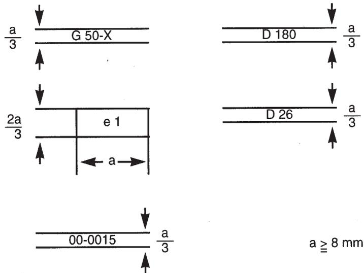
The coupling device with the EEC approval marking illustrated above is a non-standard fifth wheel coupling of Class G 50-X having a maximum permitted D value of 180 kN and a maximum permitted fifth wheel load of 26 tonnes, for which EEC component type-approval was granted in the Federal Republic of Germany (e 1) under the number 0015. The first two digits 00 indicate that this component was approved according to the original form of this Directive.
