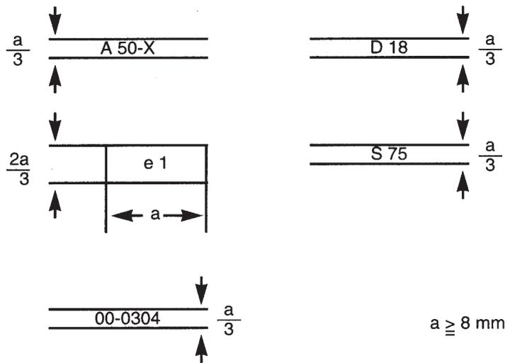
The coupling device with the EEC approval marking illustrated above is a non-standard coupling ball and towing brackets of Class A 50-X having a maximum permitted D value of 18 kN and a maximum permitted static vertical bearing load of 75 kg, for which EEC component type-approval was granted in the Federal Republic of Germany (e 1) under the number 0304. The first two digits 00 indicate that this component was approved according to the original form to this Directive.
