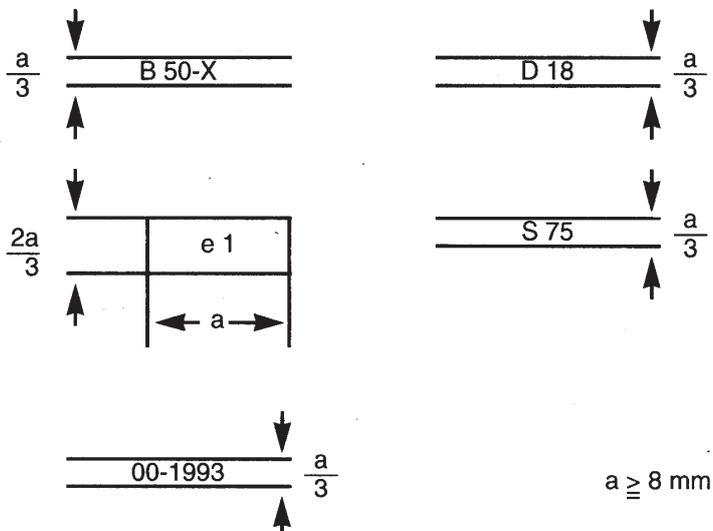
The coupling device with the EEC approval marking illustrated above is a non-standard coupling head of Class B 50-X having a D value of 18 kN and a maximum permitted static vertical bearing load of 75 kg, for which EEC component type-approval was granted in the Federal Republic of Germany (e 1) under the number 1993. The first two digits 00 indicate that this component was approved according to the original form of this Directive.
