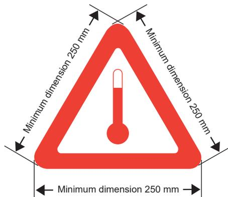
Mark for carriage at elevated temperature
