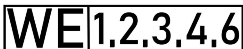
In this example, the wagon is fitted with wagon equipment 1, 3, 2, 4 and 6.
