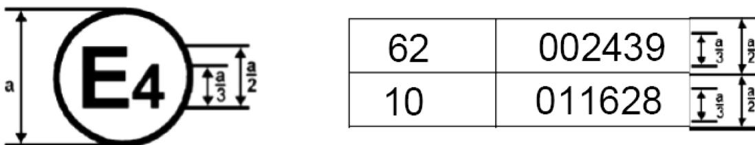
The above approval mark affixed to a vehicle shows that the vehicle type concerned has been approved in the Netherlands (E 4) pursuant to the Regulations Nos 62 and 10<sup>(1)</sup>. The approval numbers indicate that, at the dates when the respective approvals were given, Regulation No 62 had not been modified, and Regulation No 10 already included the 01 series of amendments.
