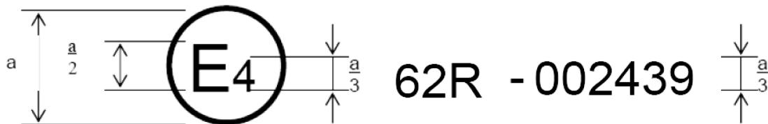
The above approval mark affixed to a vehicle shows that the vehicle type concerned has, with regard to the protection against unauthorized use, been approved in the Netherlands (E 4) pursuant to Regulation No 62 under the approval number 002439. The approval number indicates that the approval was granted in accordance with the requirements of Regulation No 62 in its original form.
