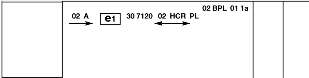
*Note:* The four examples of approval marks, models A, B, C and D represent four possible variants of the marking of a lighting and light-signalling device when two or more lamps are part of the same unit of grouped, combined or reciprocally incorporated lamps. These approval marks show that the device was approved in Germany (e1) under the base approval number 7120 and comprises:
