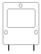
The front lights must optimise train detectability (e.g. to track workers and those using public crossings), provide sufficient visibility for the train driver (illumination of the line ahead, lineside information markers/boards, etc) by night and during low light conditions and shall not dazzle the drivers of oncoming trains.
