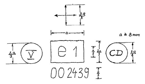
The above component type-approval mark shows that the interior material in question has been approved in Germany (e1) pursuant to this Directive (00) under the approval number 2439. The first two digits indicate that this component was approved according to the original form of this Directive. The additional symbol - indicates that this type of material has been approved according to its horizontal and vertical burning rate.
