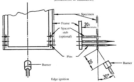
Figure 2 Burner ignition location
