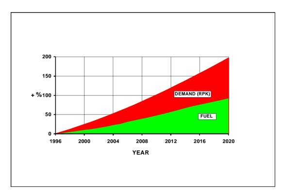
Figure 7: Growth of Air Traffic and Fuel Consumption
