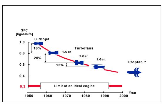
Figure 8: Engine Technology Steps and Gain of SFC
