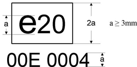
The above certification mark affixed to an engine shows that the type concerned has been certified in Poland (e20), pursuant to this Regulation. The first two digits (00) are indicating the sequence number assigned to the latest technical amendment to this Regulation. The following letter indicates that the certificate was granted for an engine (E). The last four digits (0004) are those allocated by the approval authority to the engine as the base approval number.
