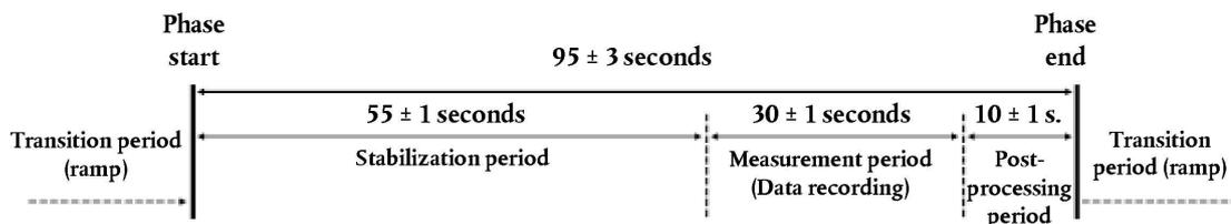
Figure 4 exemplarily illustrates the sequence of steady state measurement setpoints to be followed for the test.
