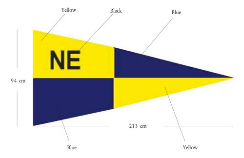
2. The boarding craft shall display one inspection pennant as indicated above. The pennant may be half scale. The pennant may be painted on the hull or on any vertical sides of the craft. When painted, the black letters "NE" can be left out.
