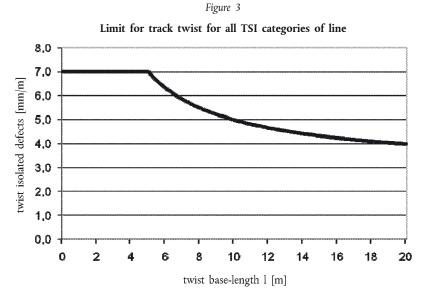
(3) (The infrastructure manager shall set out in the maintenance plan the basis on which it will measure the track in order to check compliance with this requirement. The basis of measurement shall include at least one measurement base between 2 and 5 m.
