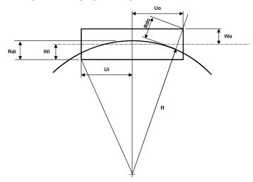
The overthrows at a point on a vehicle body is the difference between the radial distance from the track centreline to the point (Rdo or Rdi), and the lateral distance from the vehicle centreline to the point (Wo or Wi). This is calculated with the vehicle stationary.
