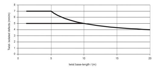
The Infrastructure Manager shall set out in the maintenance plan the basis on which it will measure the track in order to check compliance with this requirement. The basis of measurement shall include a measurement base of 3 m.
